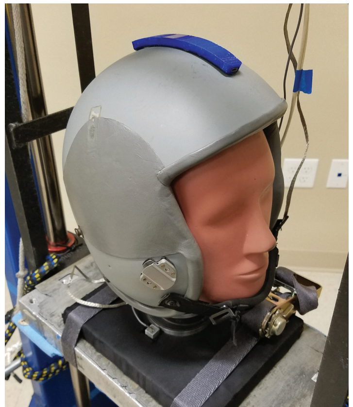
The miniature Dynamic Impact Recorder DTS is developing for the U.S. Air Force will measure forces that pilots may experience during an emergency ejection maneuver. The unit (shown as a prototype on the helmet) will collect data used to improve safety gear for USAF pilots.
