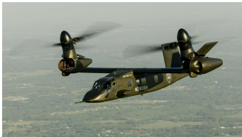
Bell's V-280 Valor tiltrotor won the US Army's Future Long-Range Assault Aircraft (FLRAA) competition. (Bell), East West is making the Troop and Gunner Seats
